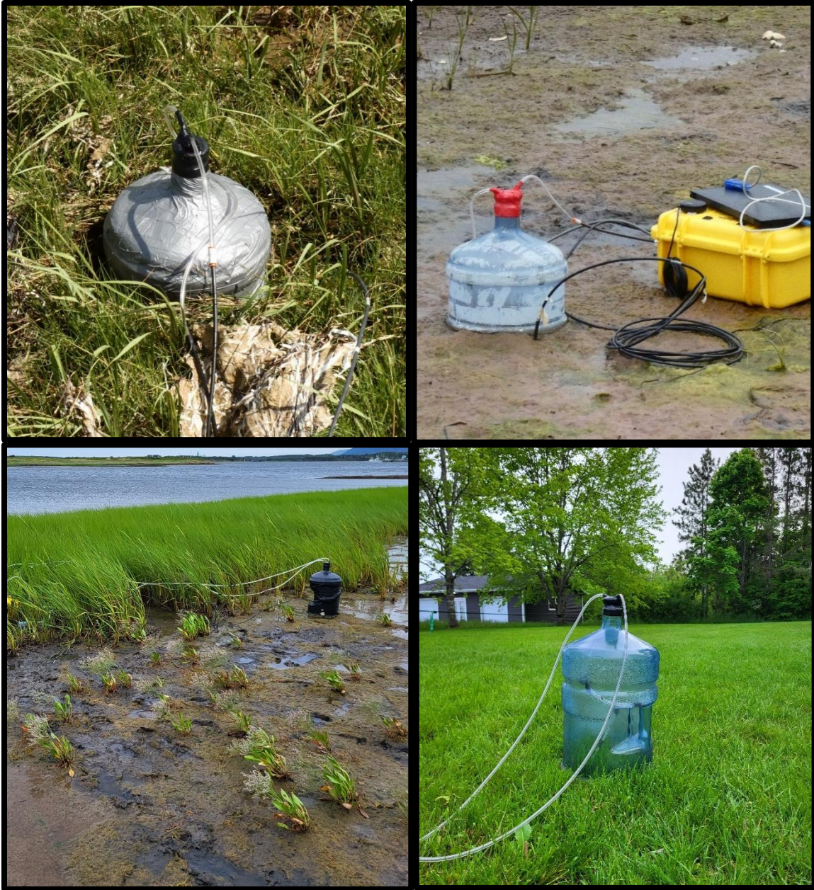
Figure 8. Four variations of simple soil gas chamber. The upper left image shows the ‘ small-dark chamber ,’ which is 8.3439 L in volume and 0.05726 m 2 in basal surface area. The upper right image shows the ‘ small-light chamber ,’ which has the same dimensions. The lower left image shows the ‘ large-dark chamber ,’ which is 17.599 L in volume and 0.05726 m 2 in basal surface area. The lower right image shows the ‘ large-light chamber ,’ which is 17.349 L in volume and 0.05683 m 2 in basal surface area. Chambers were made of polycarbonate. Black or red electrical tape attaches vinyl tubing to the chambers and functionally block exterior air exchange. Black electrical tape and duct tape were also used to block light from entering the dark chambers. During a soil gas measurement, one of these chambers would be attached to a portable gas concentration analyzer, using ‘quick-connect tube fittings,’ and placed on a soil surface.
